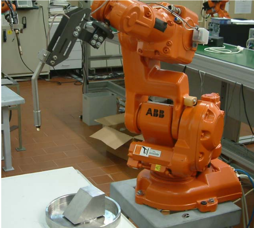
Robot and welding test case
