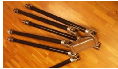
Fig. 3. Picture showing arm links dimensioned for industrial usage (with wrist mount).
