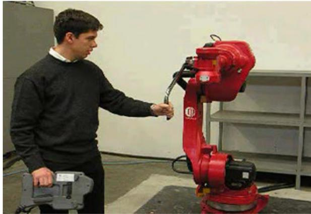
Figure 11 Manual Guidance of a COMAU NS-16 robot
