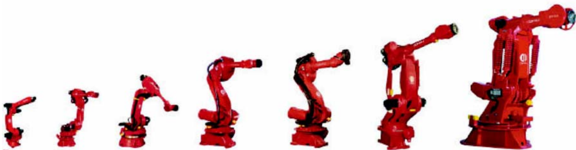
Fig. 2 – Comau SMART robot range: from 6 up to 800 Kg payload
